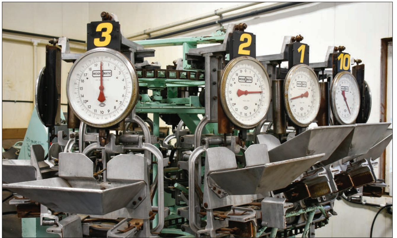
The machine for barring 10-pound bags still requires human assistance to get the final product
