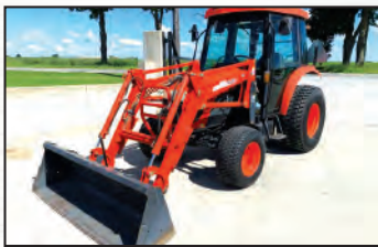
Kioti DK55 55hp Duedong 2.2L 4-Cyl Eng, 12 Gear Trans, 540 PTO, 2-Hyd Rem., Turf Tires, KL551 Loader, 1580 hrs ..... $35,000
