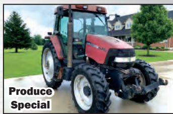
Case MX80C 2002 with 8236hrs, 84hp 4L Eng, 4-Range 4PS Creeper Trans, 540-1000 PTO, 3-Hyd Remotes, Zuidberg Front Hitch with 1-Hyd Remote. $27,000
